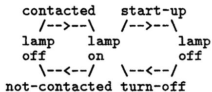
Fig. 7 The exported state-transition diagram of the oil-pressure-indicator-lamp
