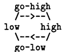
Fig. 6 The state-transition diagram of the oil-pressure-sensor
