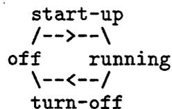
Fig. 4 The state-transition diagram of the start-engine.
