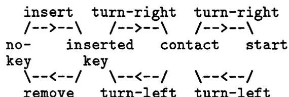
Fig. 3 The exported state-transition diagram of the ignition-lock.
