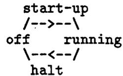
Fig. 5 The state-transition diagram of the engine.
