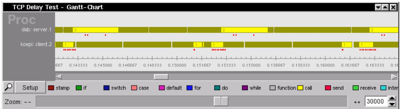
Figure 10: Interrupt Occurrences with Nagle Algorithm Disabled
