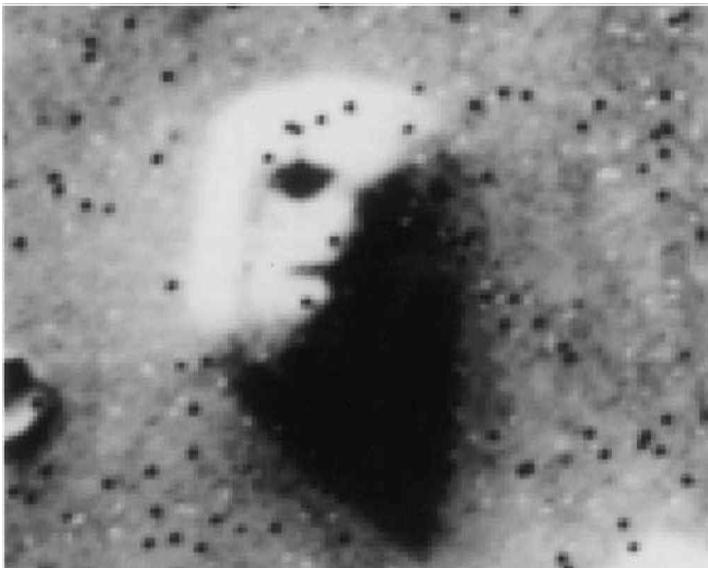
Fig. 1. The famous "Face on Mars" picture, cropped from the original JPL Press release photograph (Viking 1-61, P-17384 (35A72), July 31, 1976). Note the fortuitous black pixel "bit-hit" that suggests the presence of a left "nostril." The black and white pixels seen in this picture are examples of so-called "salt and pepper" noise that was later removed using adjacent pixel average techniques. Feature is 1.5 – 2 km across. Courtesy NASA/JPL.
