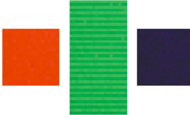
Figure 2: Raw Bayer image data of a constant background showing variation (banding) in the green data
