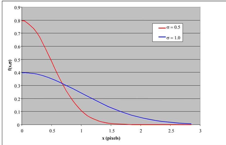
Figure 3: Filter curves generated with equation (1)
