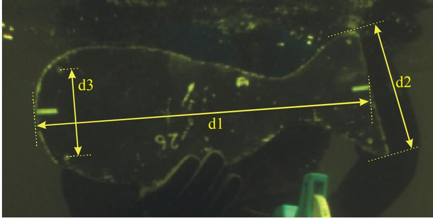
Figure 5: Test object for underwater measurement validation showing dimensions measured
