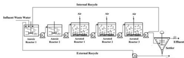
Fig. 1. Layout of the BSM1 benchmark simulation plant
