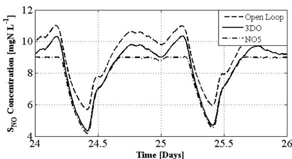
Fig. 3. Nitrate nitrogen concentration in the last aerated reactor.
