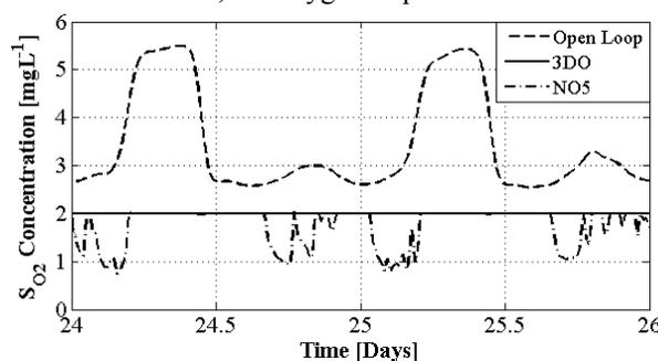
Fig. 4. Oxygen concentration in the last aerated reactor.
