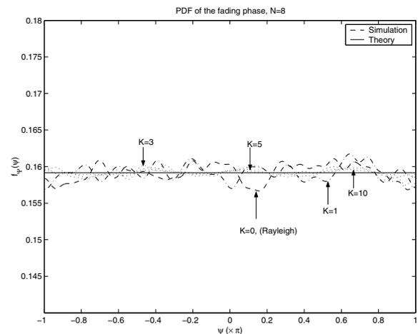
Fig. 4. The PDF of the fading phase  $\Psi(t)$ .
