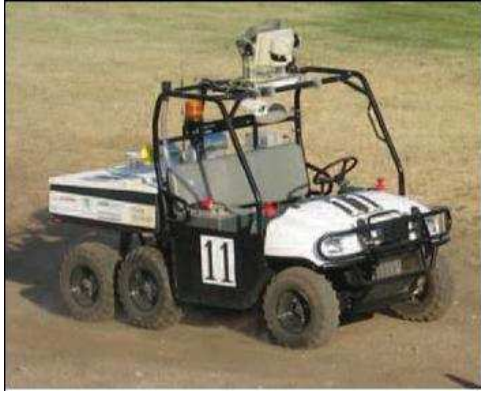
Figure 13: The Overbot, the autonomous ground vehicle at Autonomous Systems Lab at UCSC.
