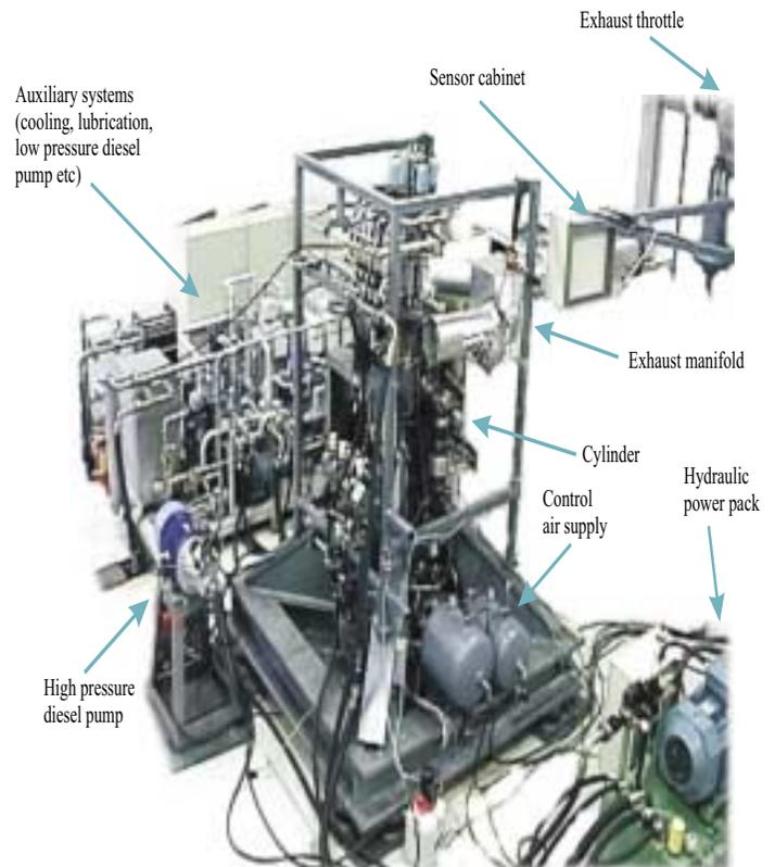
Fig. 4. Picture of test cylinder test unit.
