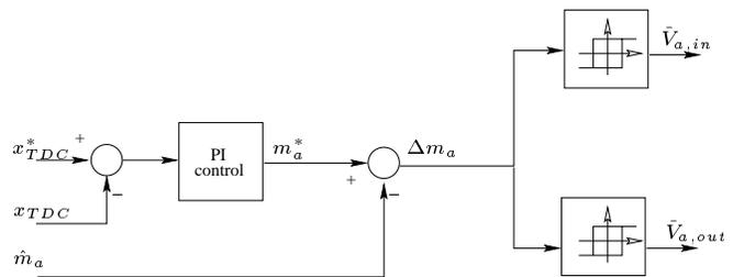
Fig. 10. Block diagram with TDC controller.
