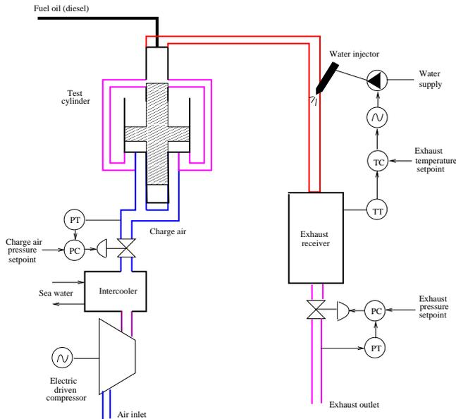
Fig. 5. Overall setup for single cylinder test unit.
