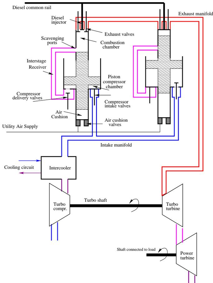
Fig. 1. Sketch of multi-cylinder free-piston engine.
