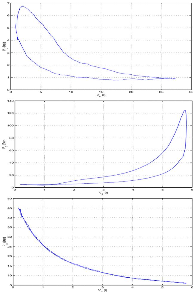
Fig. 2. Experimental pV-diagrams corresponding to about 20 % load: Piston compressor, combustion chamber and air cushion.
