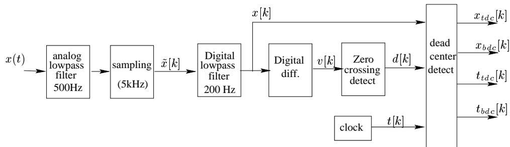
Fig. 8. Algorithm for robust detection of piston dead centers.
