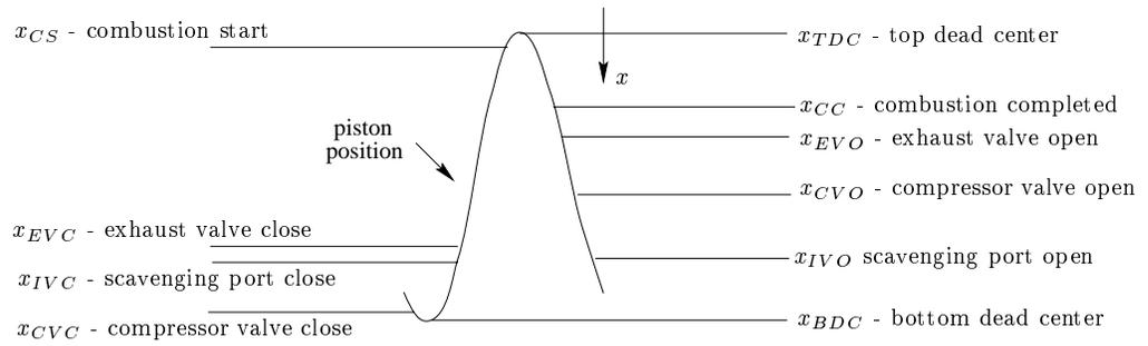
Fig. 3. Main events during the two-stroke free-piston diesel cycle.
