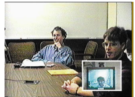
Figure 5. The Virtual Window camera control system in operation. The larger images represent the view received by the remote participant, while the small inset images represent the appearance of the participant on a local video monitor. The motorized camera appears at the top of the video monitor.
