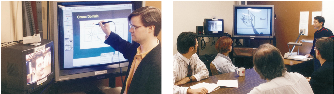
Figure 1. a) The digital whiteboard in use. The design being sketched is visible to people in the room and to the telepresent attendee, whose image appears on the smaller monitor. b) The speaker (top-right) is illustrating a diagram in the document camera. The document is displayed on the large video monitor and is also visible to the telepresent attendee.
