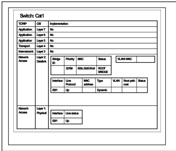
Figure 1: Switch State Model Diagram
