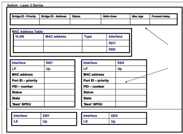
**Figure 8: Switch – MAC address table and STP tables**
