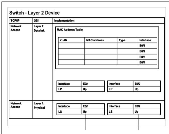
**Figure 7: Switch and MAC address table**
