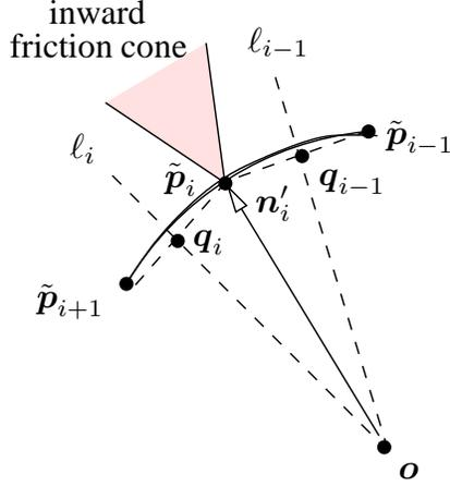
**Figure 14:** Estimation of the normal at displaced node  $\tilde{p}_i$  in contact with a point finger exerting force.
