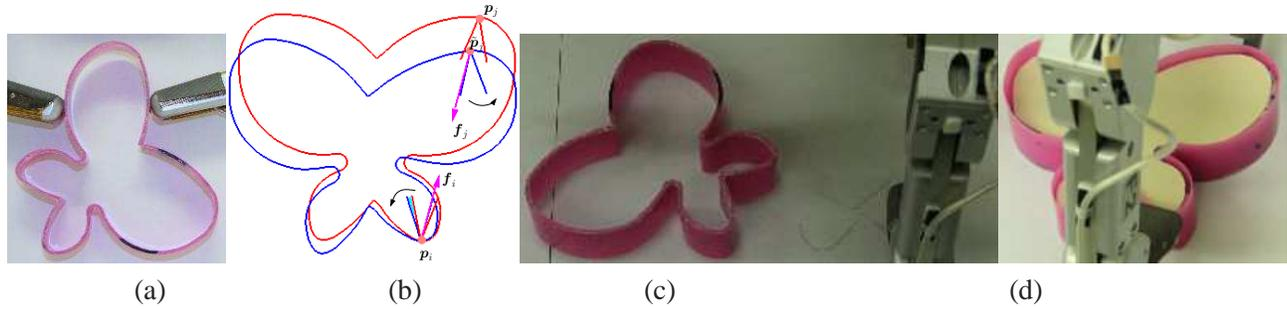
**Figure 12:** Grasp failure due to deformation: (a) attempt with a 15% relative squeeze; (b) contact forces out of the friction cones; (c) escape of the object; (d) success at grasping a “rigid” identical shape with the same placement.
