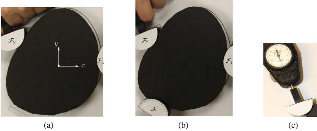
**Figure 10:** Experiment on adversary finger resistance: (a) grasp of a foam rubber object; (b) its resistance to a translating finger  $\mathcal{A}$ ; (c) force meter (from Ametek Hunter Spring) attached to a finger for force measurement.
