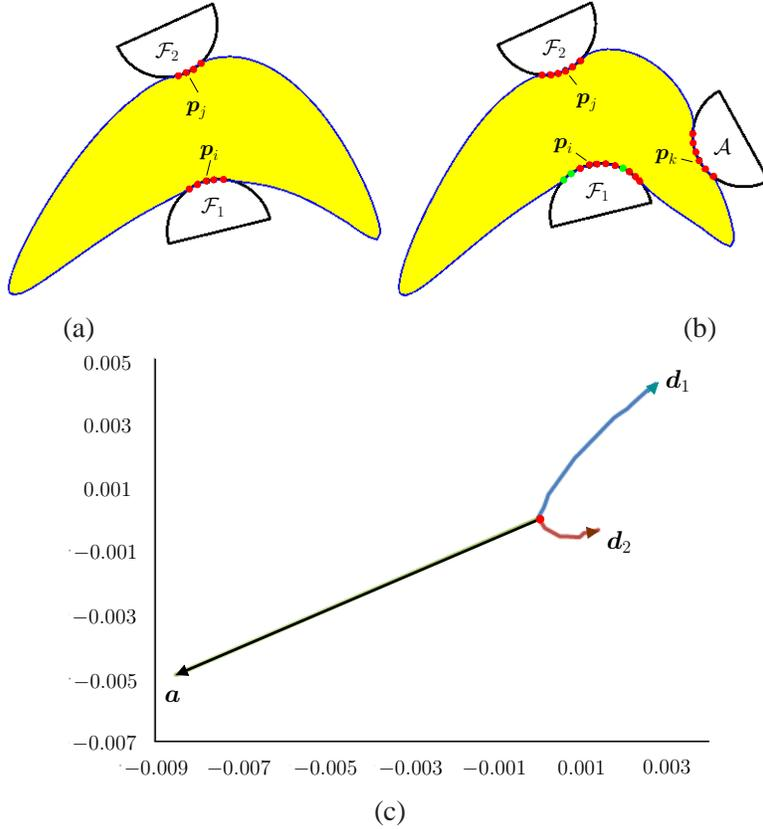
**Figure 9:** Adversary finger resistance with frictional segment contacts: (a) the shape from Figure 8 grasped via a pure squeeze at the same initial contact nodes; (b) successful resistance to the same adversary finger disturbance as in Figure 8; and (c) trajectories of the three fingers during the resistance. Sticking contacts are in red, and sliding contacts are in green.
