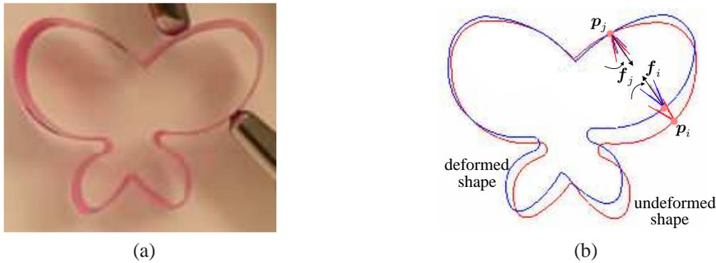
**Figure 13:** Rotations of two contact friction cones make the grasping forces more aligned in (a) experiment and (b) corresponding simulation, where the arrows indicate the rotation directions. The contact forces are collinear and opposed.
