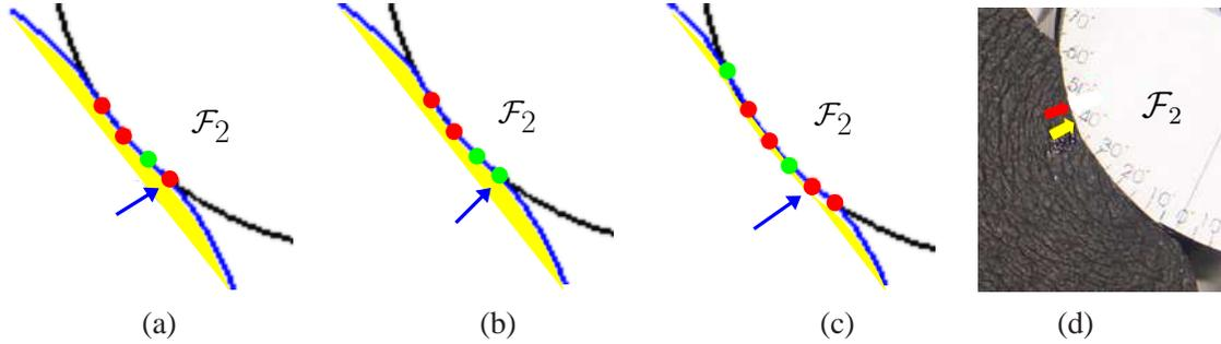
**Figure 5:** Transitions of a contact from stick (a) to slip (b) to slick (c). Here (a) and (b) are the simulation results over the second object in Table 2 that correspond to its entries (2, 3) and (3, 3), respectively. In (c), the contact has stopped sliding, as also indicated by the experiment in (d).
