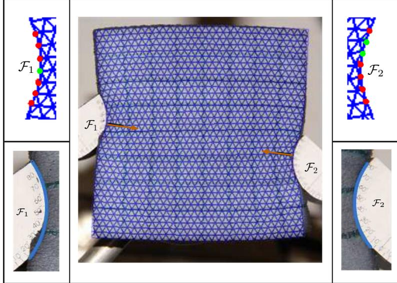
**Table 1:** Grasped foam rubber square superposed by its deformed mesh (center): the contact segments from simulation (row 1) composed of sticking nodes (red) and sliding nodes (green); the contact segments in the experiment (row 3) enlarged from the center image.
