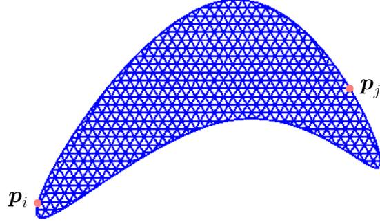
**Figure 2:** Meshed object with 517 nodes, including 112 on the boundary.
