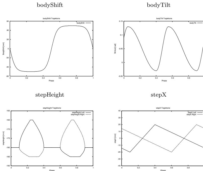
**Figure 1.** The walk step trajectories are in total described by 16 parameters, which are responsible for their shapes and proportions. The shown values are taken from the *B-Human walking engine*, which serves also in our team and was originally developed for a slightly modified Kondo KHR-1 robot.
