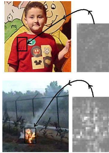
Fig. 3. Comparison of spatial variations of fire-colored regions. Flame(bottom-left) have substantially higher spatial variation(bottom-right) compared to an ordinary fire-colored region.
