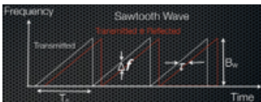
Figure 2: FMCW Principles - Sawtooth Wave Sweep.
