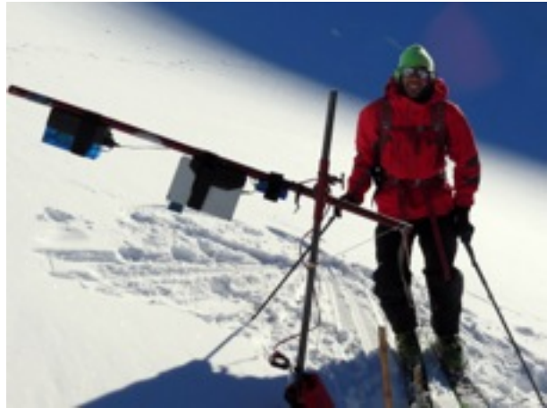
Figure 5: Third generation MiniFMCW Snow Radar Systems. In the left (blue housing) the 25 GHz radar, in the center (white housing) the 10 GHz radar. Remote installation at Cerro Cautin, Malcalhue, Chile.
