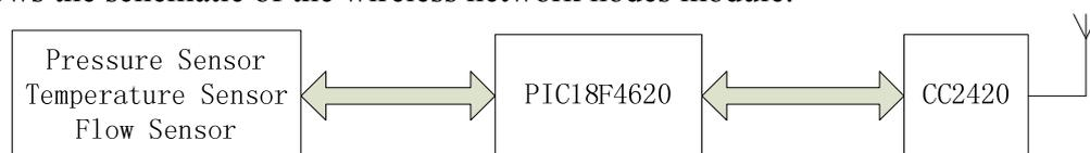
Fig.1 The Schematic of Nodes Module
