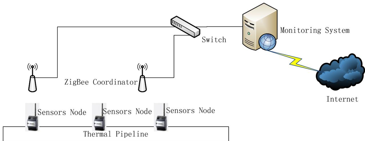
Fig.2 Design of Wireless Sensors Network
