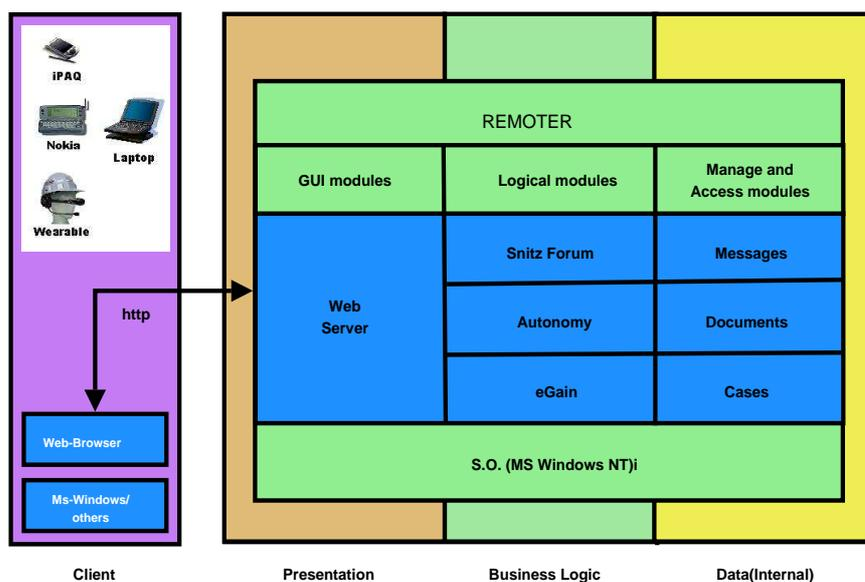
Figure 9: Remoter tree-tier Architecture.
