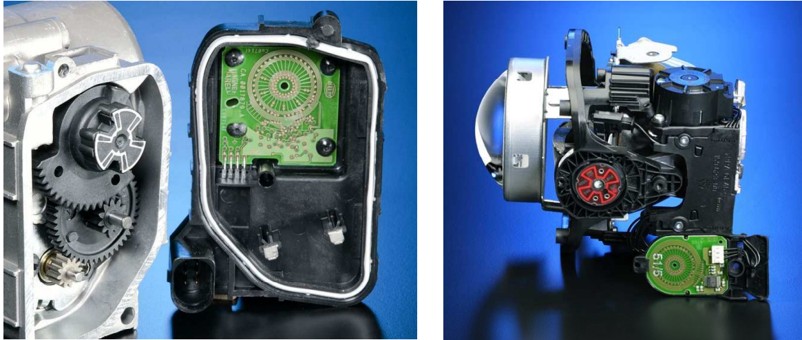
Fig. 24 CIPOS-Sensors in Throttle-Flap and a Headlamp Swivelling Module
