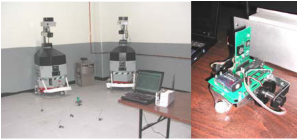
Figure 3: CyberGuard SR2/ESP, inexpensive Rovers, and MICA Xbow motes on the DIAL lab floor
