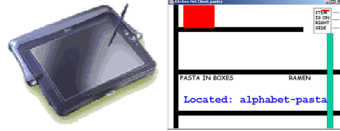
Figures 2a and 2b. The Kitchen-Net interactive prototype. PDAs, displaying the Kitchen-Net client program and networked on a wireless LAN, replaced the paper screens.
