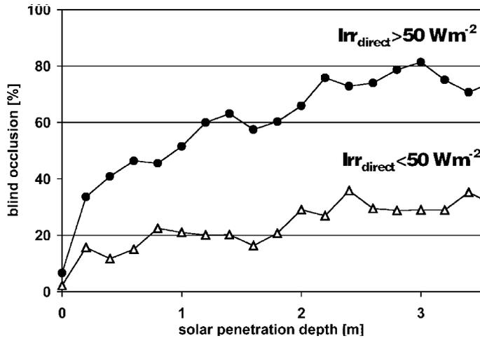
**Figure 7** Mean blind occlusion for different solar penetration depths for all the investigated offices for all occupied times. The dots (triangles) correspond to times with  $I_{direct}$  solar irradiances above (below)  $50 \text{ W/m}^2$
