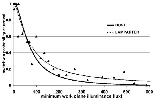
**Figure 1** Comparison of the switch on probabilities upon arrival found by Hunt in the Lamparter building. The triangles correspond to measured switch-on probabilities in the Lamparter building
