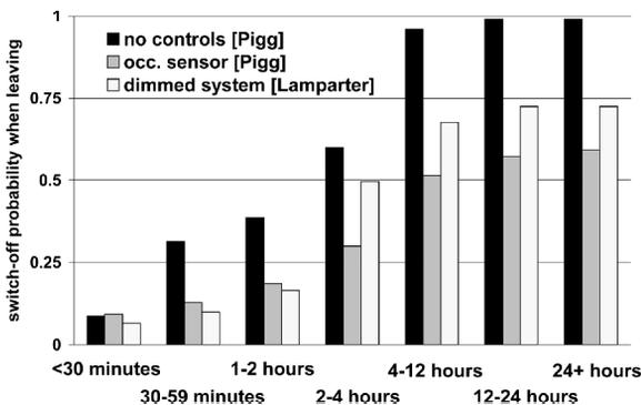
**Figure 2** Comparison of measured switch-off probabilities for different times of user absence for a lighting systems without controls and with an occupancy sensor (according to Pigg), as well as for the dimmed, indirect system from the Lamparter building
