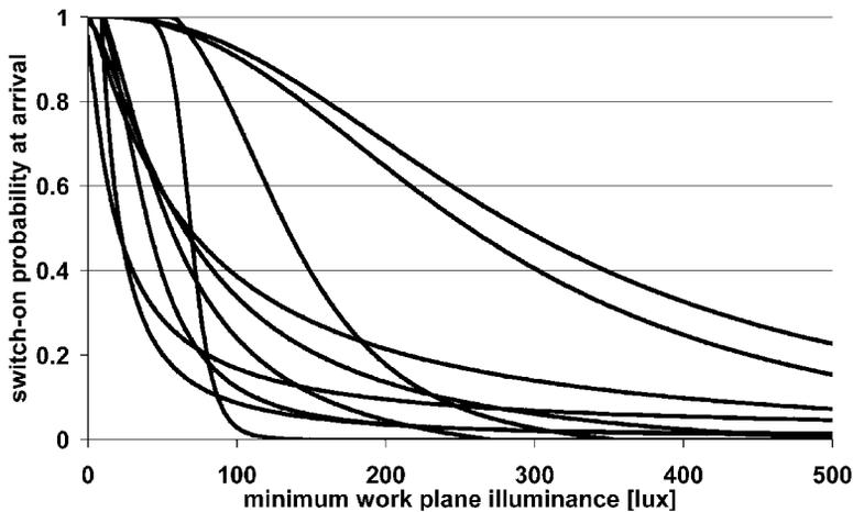
**Figure 5** Individual switch-on probabilities as a function of work plane illuminance in all offices
