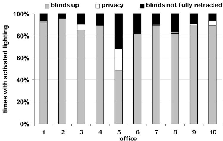
**Figure 8** Status of the venetian blinds during hours when the offices were occupied and the lighting was activated
