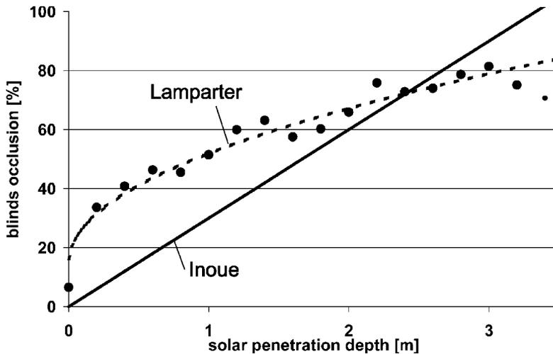
**Figure 3** Mean blind occlusion for different solar penetration depths for all investigated offices, for the occupied times when the direct solar irradiance was above  $50 \text{ W/m}^2$ . The straight line corresponds to Inoue's fit, whereas the parabolic graph (-) is fitted to the Lamparter data. The parabolic fit corresponds to  $y = 15 + \sqrt{-0.116 + 1359x}$  with  $y =$  blind occlusion (%) and  $x =$  solar penetration depth (m)
