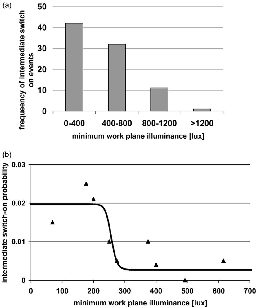
**Figure 6** (a) Histogram of intermediate switch-on events ordered by their pertaining minimum indoor illuminances. (b) Intermediate switch-on probability for all 10 offices based on 5-min-time-step-intervals
