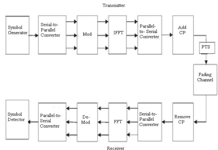
Figure. 2 Block diagram of OFDM System
