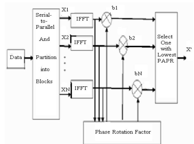
Figure.5 Block Diagram of Partial Transmit Sequence
