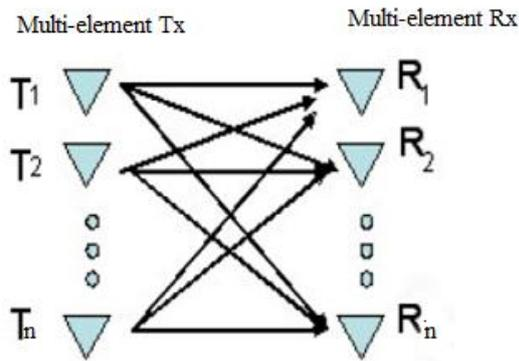
Figure.3 Structure of MIMO
