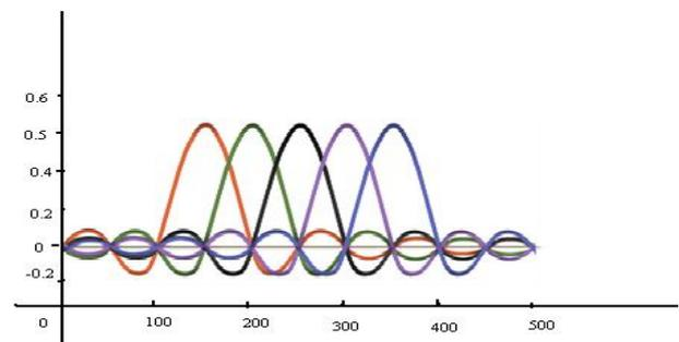
Figure.1 OFDM Spectrum
