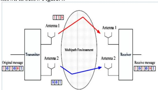
Figure.4 A 2x 2 MIMO systems with a spatial multiplexing scheme
