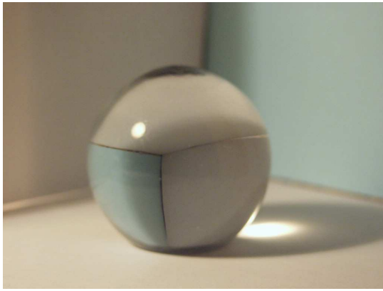
Fig. 2. Photograph of caustics from a spherical glass paper weight using a desk lamp to emulate directional spotlighting. The caustics are formed on rough paper placed underneath the refractive object.
