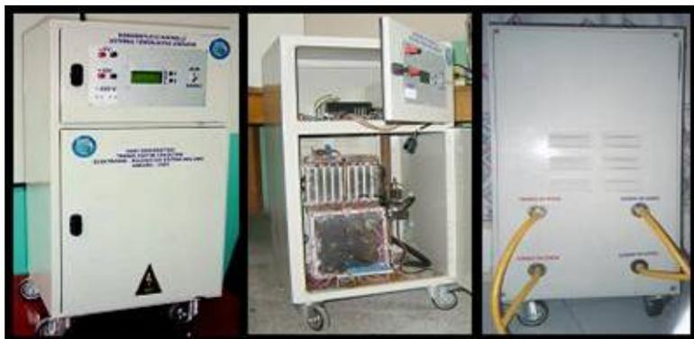
Figure 2. Microcontroller controlled geothermal thermoelectric generator
