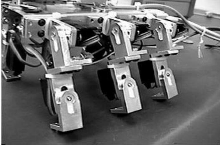
**Figure 7.** Legs of hexapod prototype.
