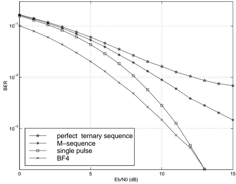
Figure 1: Short sequences BER performance for an exponential channel profile and supersymbol path delays.
