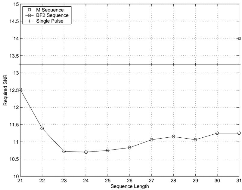
Figure 6: Required SNR vs sequence length for  $BER=10^{-3}$  (Increasing ISI experienced with a decrease in zero padding for beamforming sequences.)
