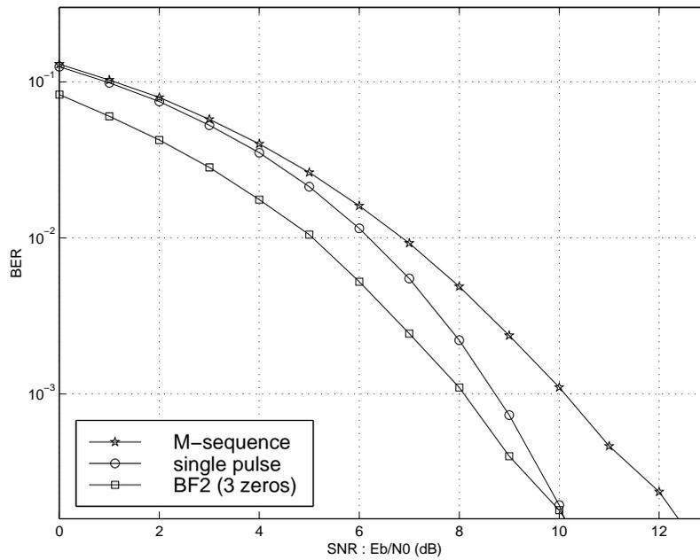
Figure 2: Short sequences BER performance for an exponential channel profile and subsymbol path delays: PAR optimized sequences.
