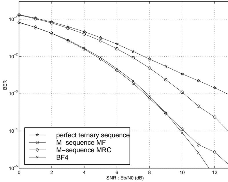
Figure 3: Short sequences BER performance for the channel based on [10].
