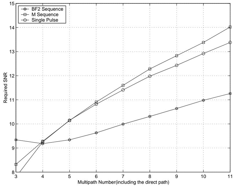
Figure 5: Required SNR vs number of multipath components for  $BER=10^{-3}$
