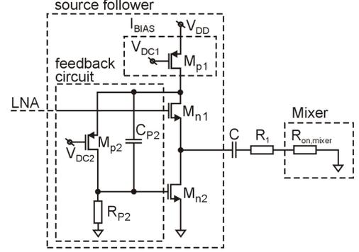
Figure 3. Simplified schematic of the source follower
