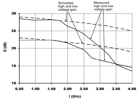
Figure 8. Voltage gain of the receiver RF front-end as a function of RF frequencies
