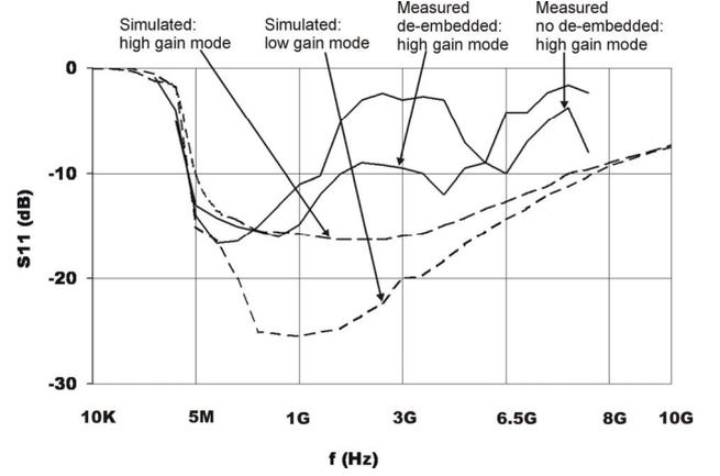
Figure 7. S11 of the receiver RF front-end
