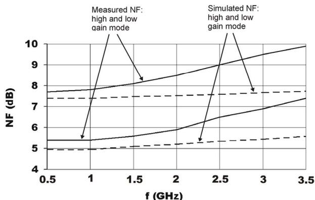
Figure 9. NF of the receiver RF front-end
