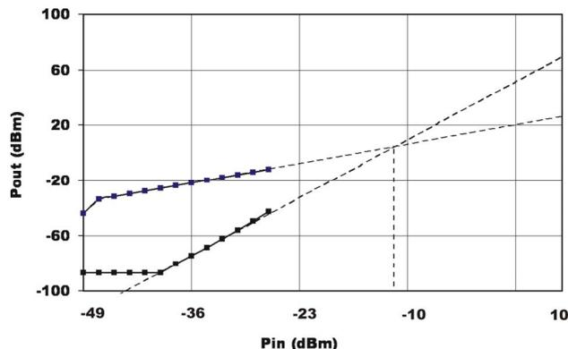
Figure 10. Measured IIP3 in the high gain mode
