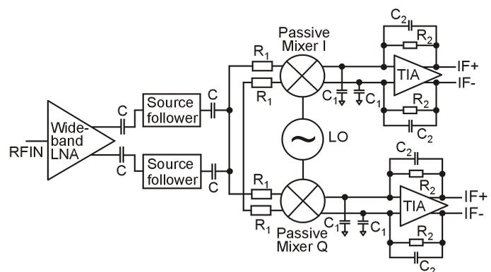
Figure 1. Wide-band receiver front-end
