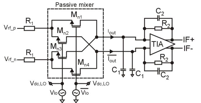
Figure 4. Simplified schematic of the passive mixer
