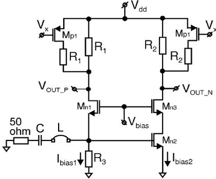
Figure 2. Simplified schematic of the wide-band LNA
