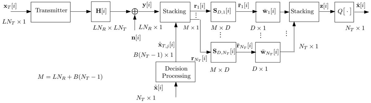
Fig. 2. Proposed MIMO reduced-rank decision feedback equalization structure.
