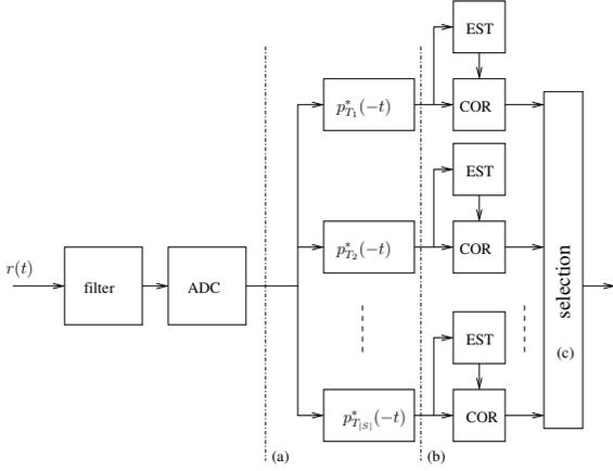
Fig. 1. Generic multi-rate receiver consisting of a bank of matched filters parameter estimation (EST) and correction (COR)
