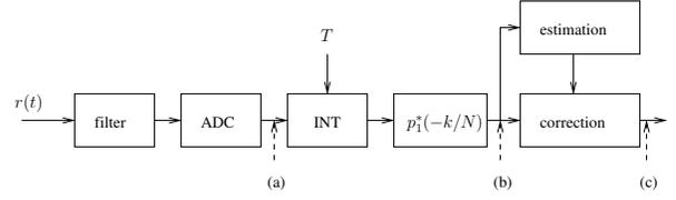
Fig. 2. Low-complexity multi-rate receiver consisting of an interpolator (INT), followed by a fixed matched filter. The interpolator requires knowledge of  $T$ .
