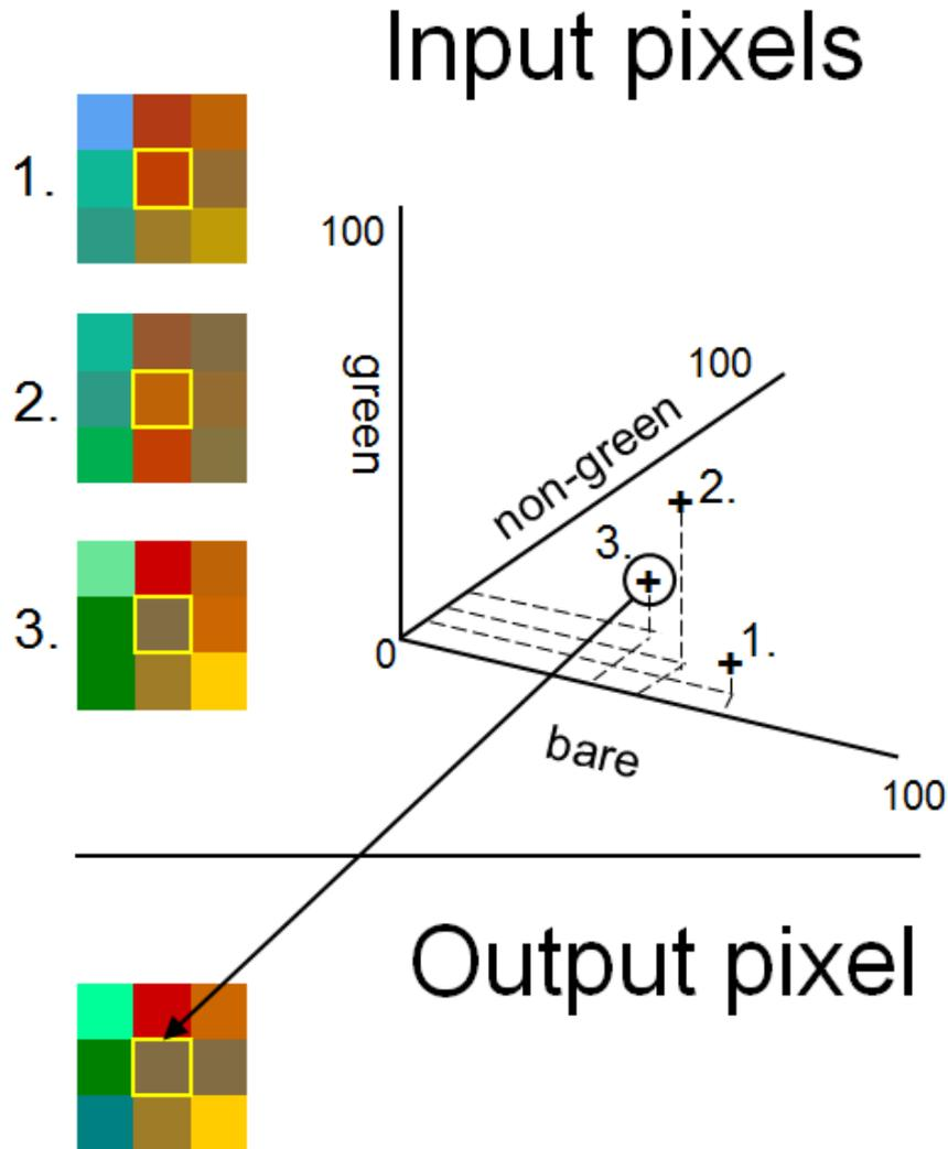
Figure 3: The method used to select the pixel for the output image from the available input pixels. For each pixel the distance to all other pixels is calculated in feature space, using the sum of squared differences. The pixel with the smallest distance is considered to be closest to the centre of the data cloud, and is chosen as the output pixel. The output pixel is the medoid of the input pixels.
