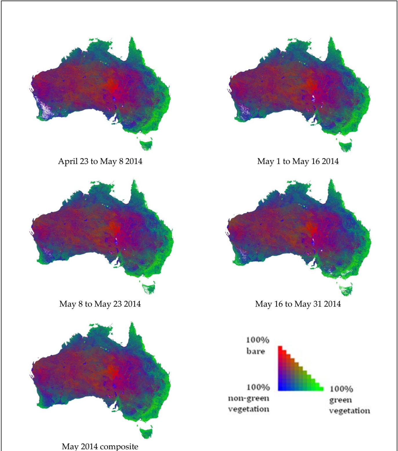
Figure 2: A compositing example. The cover image for May 2014 has been created from four fractional cover images. There may be overlap with previous and following months in the monthly composite. The choice of input images is biased so that the monthly image is available soon after the end of the month.
