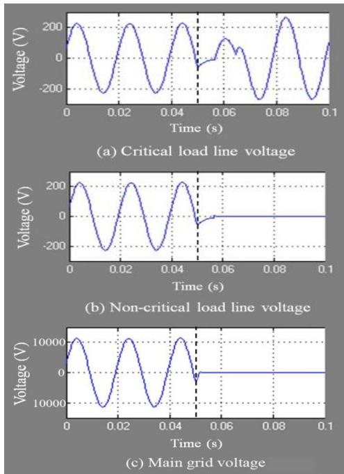
**Fig. 5.** Simulation results during intentional islanding. (a) Line to line voltage across critical load at 'C', (b) Line to line voltage across the non-critical load at 'D', (c) Line to line voltage at breaker 'A'.
