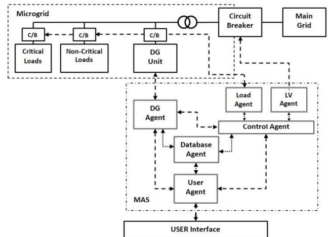
Fig. 2. Dual layered MAS architecture
