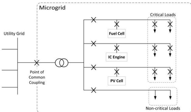
Fig. 1. Conceptual model of a microgrid
