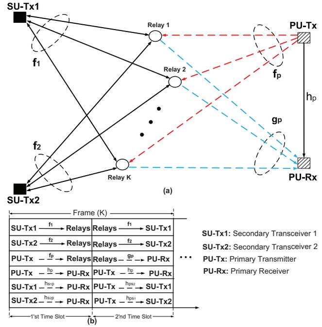
Fig. 1. (a) A proposed cognitive two-way relay network; (b) channel and interference links.
