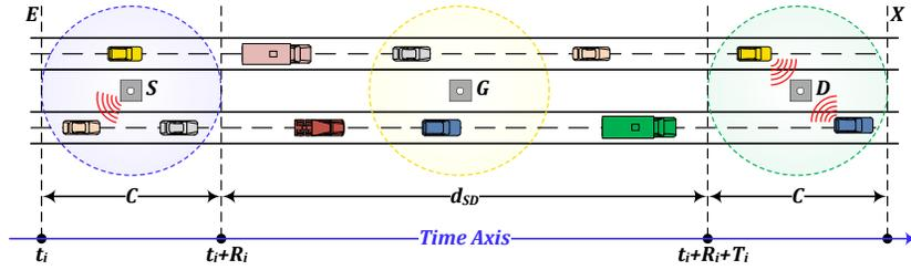
Fig. 1. Two-hop vehicular intermittently connected network scenario.
