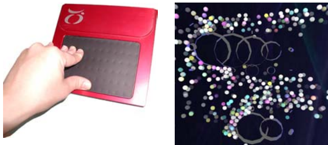
Figure 4: Applying pressure to the MTC Express (left) and resulting obstructions (right)
