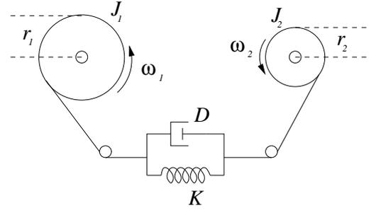
Fig. 1. Linear model for web-winding system.
