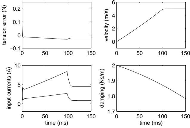
Fig. 4. Velocity ramp-up maneuver—modified controller.
