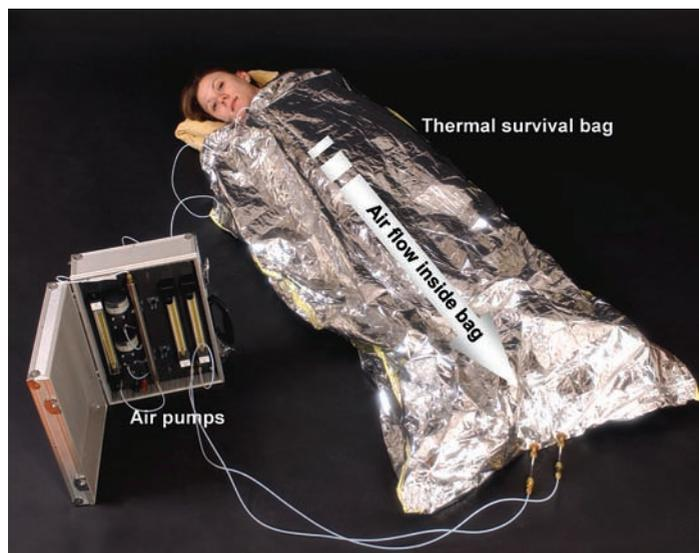
Figure 1. ‘Air entrainment’ set-up using a Lifesystems™ thermal bag (2.4 m x 09 m) to collect volatile odours from human volunteers.
