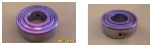
Figure 2: Inner race fault and outer race fault
