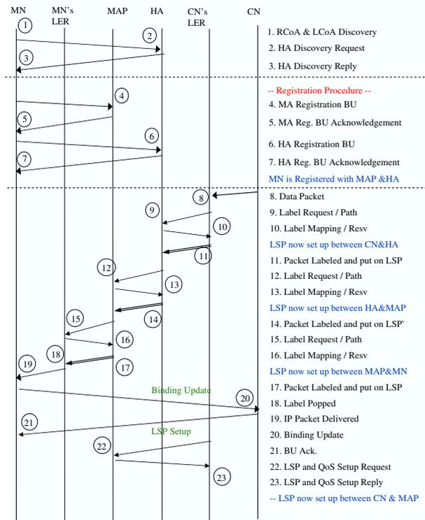
Fig. 4. MPLS data only - CN initiated communication.
