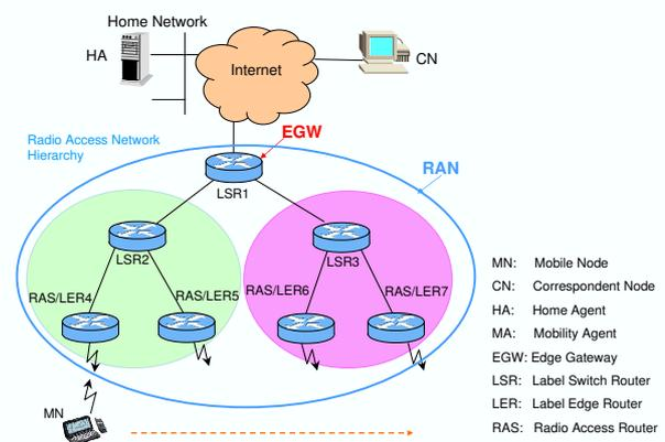
Fig. 1. Mobile MPLS Radio Access Network
