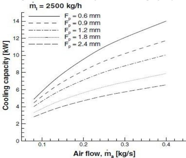
Fig.5 Effect of Fin density (affecting air flow) on cooling capacity
