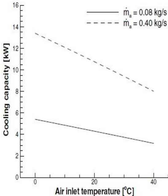
Fig.4 Effect of Air inlet temperature on cooling capacity
