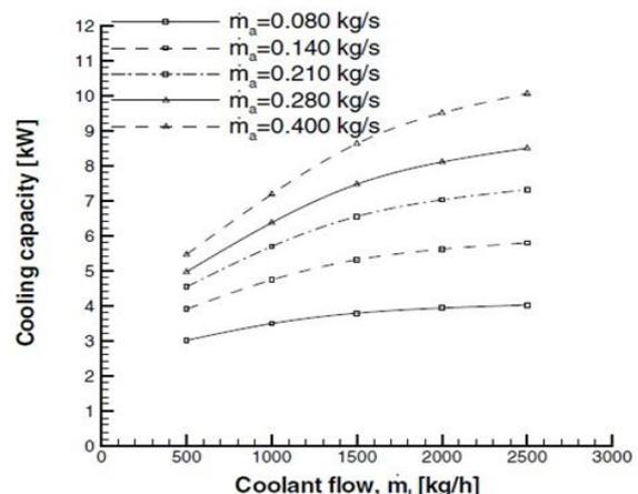
Fig.3 Effect of Coolant Flow on cooling capacity
