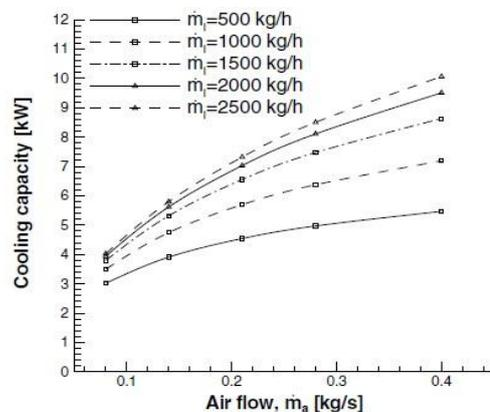
Fig.2 Effect of Air Flow on cooling capacity
