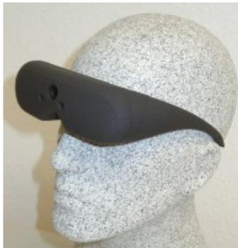
Figure 2: A video see through HMD. Picture from <http://www.vrlogic.com/>
