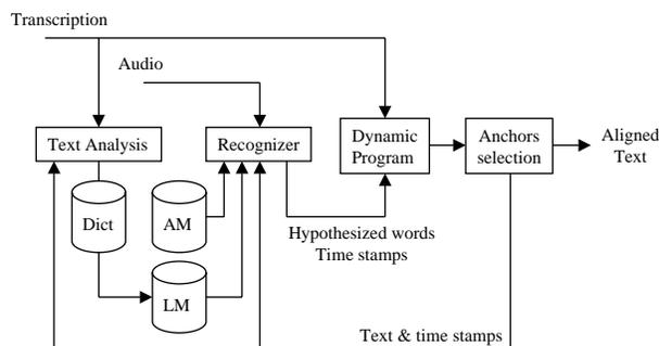
Figure 1: Block diagram of the aligner program.
