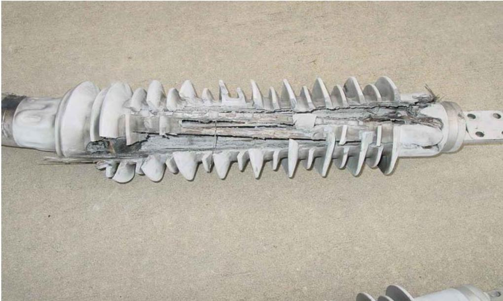
As mentioned earlier, one of the hazards of a silicon carbide arrester not venting properly can result in an explosion of the device. The failure of the arrester and the expulsion of the porcelain can result in damage to other apparatus due to shrapnel from the arrester. Several times bushings have been damaged, not by the fault, but by shrapnel from the failed arrester.
