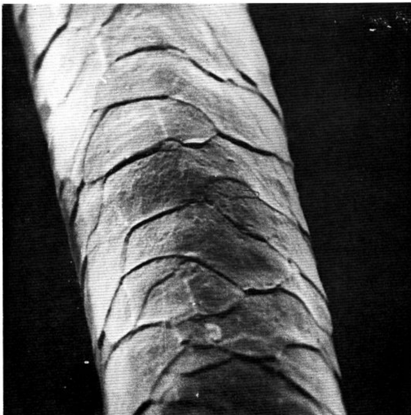
Figure 6. Scanning electron micrograph of intact mohair. Magnification, 2750
