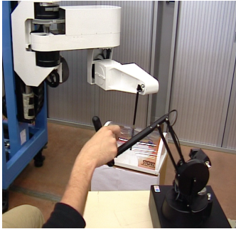
Fig. 1. Experimental setup. D2M2 robot tele-controlled by the Phantom for robotic surgery. The medical instrument has 40 [cm] height.
