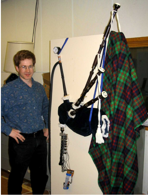
Figure 4. Garth Zeglin with McBlare shortly before its debut at the Robotics Institute’s Twenty-Fifth Anniversary. Bagpipes are mounted on a display board that conceals the pump and additional electronics.
