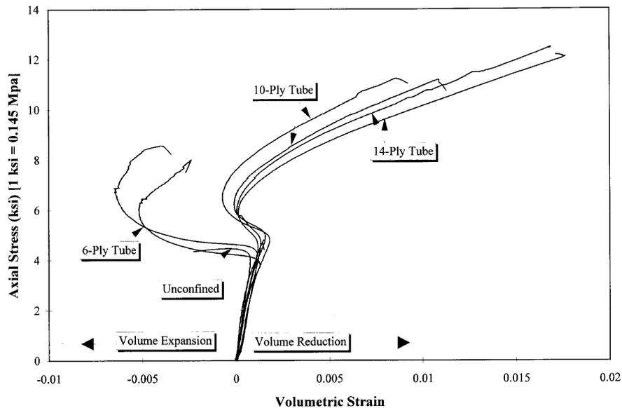
Figure 4. Axial stress–volumetric strain of FRP-encased concrete
