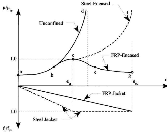
Figure 9. Schematic dilation curves for steel-encased and FRP-encased concrete
