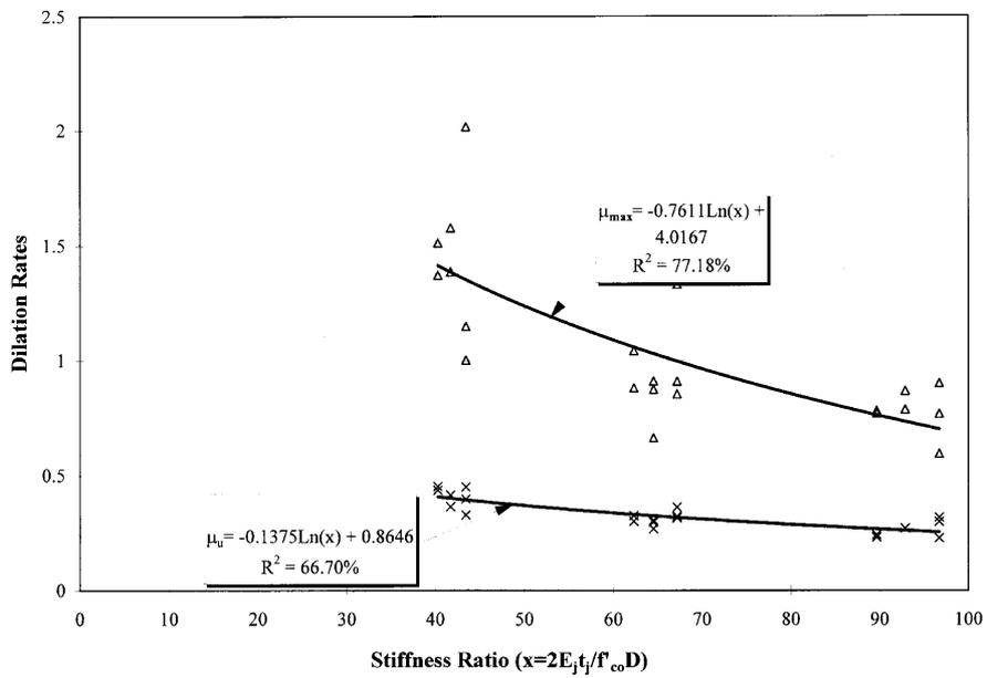
Figure 7. Effect of jacket stiffness on the peak and ultimate dilation rates
