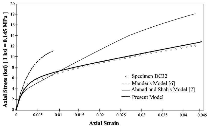
Figure 11. Comparison of confinement models for concrete-filled FRP tubes
