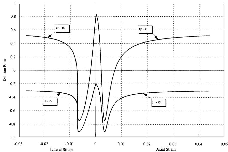
Figure 8. Lateral and volumetric dilation rates ( $\mu$  and  $\Psi$ )
