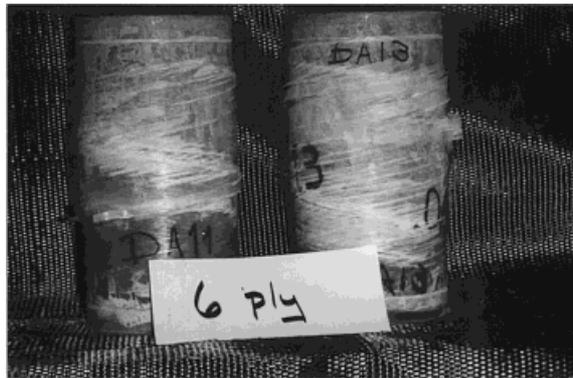
Figure 2. Typical failure for six-layer specimens
