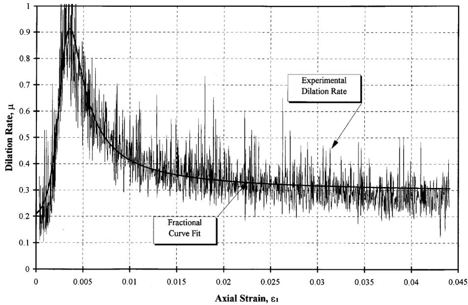
Figure 5. Typical dilation rate for FRP-encased concrete
