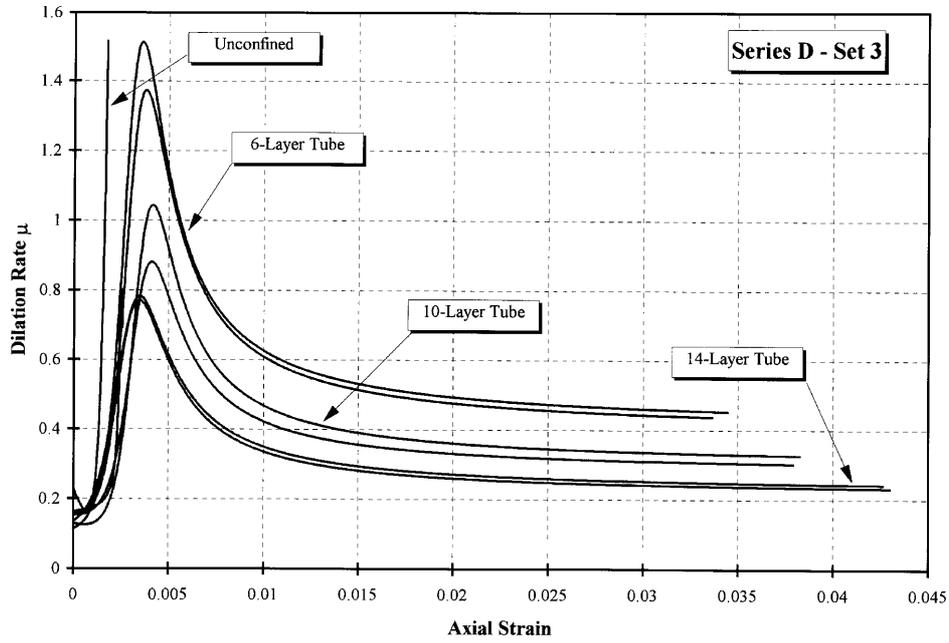
Figure 6. Effect of jacket thickness on dilation rates
