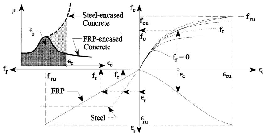
Figure 10. Schematic confinement modelling for FRP-encased concrete
