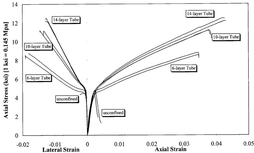
Figure 3. Stress-strain response for FRP-encased concrete
