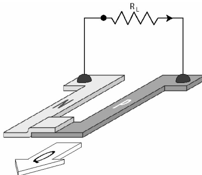
Figure 3.1 *The principle of a printed thermocouple*
