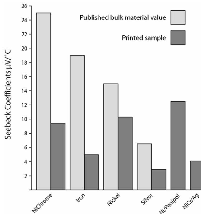
Figure 5.1 *Published bulk material Seebeck coefficients compared to those of printed samples*
