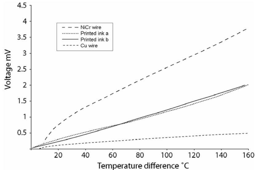
Figure 5.2 *Generated Seebeck voltages of two printed and two standard thermoelements*
