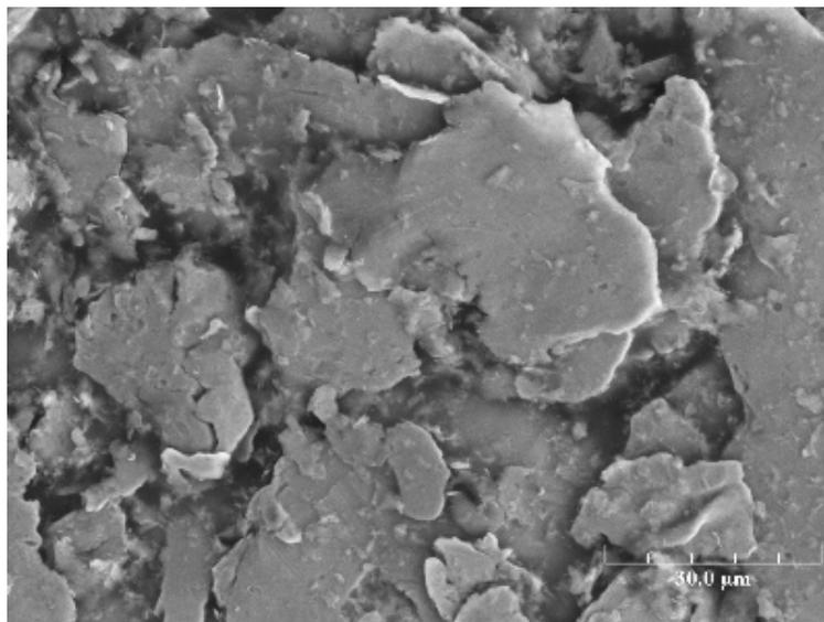
Figure 3.2 *Printed NiCr track -1000x magnification*
