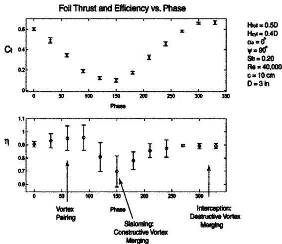
FIG. 6. The thrust coefficient  $C_t$  and efficiency  $\eta$  of a flapping foil within the wake of a vortex-shedding cylinder, plotted here as functions of the phase angle between the foil motion and the cylinder motion.
