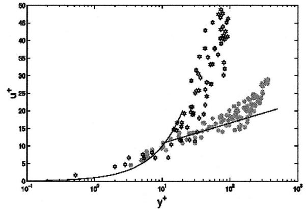
FIG. 1. The average velocity profiles for swimming and non-swimming cases. The solid lines show the “law of the wall.”
