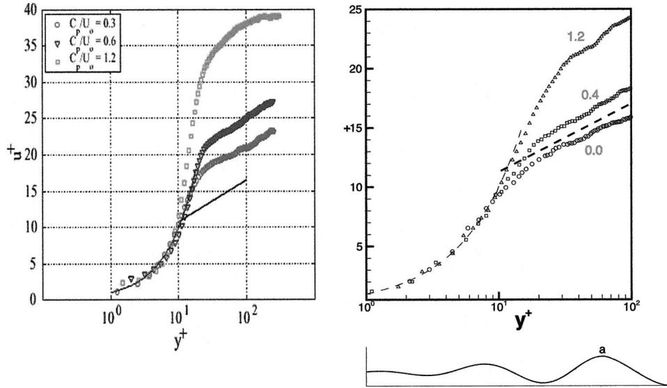
FIG. 4. Comparison between DPIV data at  $Re = 10^6$  (left) and direct numerical simulations at  $Re = 6,000$  (right).
