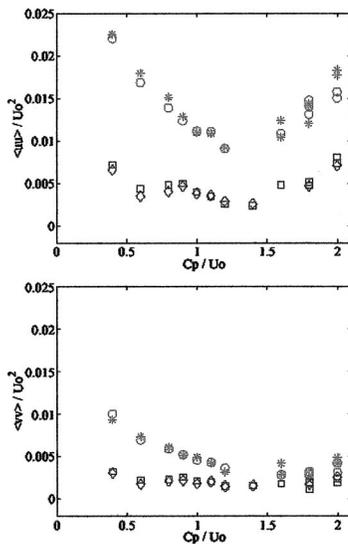
FIG. 5. The intensity of the horizontal (upper figure) and the vertical (lower figure) component of the velocity calculated from ensemble averaged LDV records obtained 4 mm under the mat boundary at piston #5.
