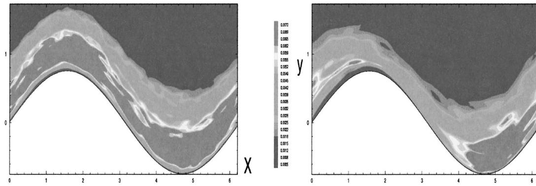
FIG. 2. The turbulence intensity along the length of a flapping plate for  $c/U = 0.40$  (left) and  $c/U = 1.2$  (right).
