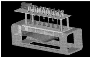
FIG. 3. The experimental apparatus to generate the wave motion.
