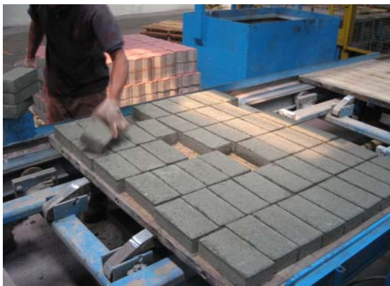
Figure 10: Finished pavers checking
