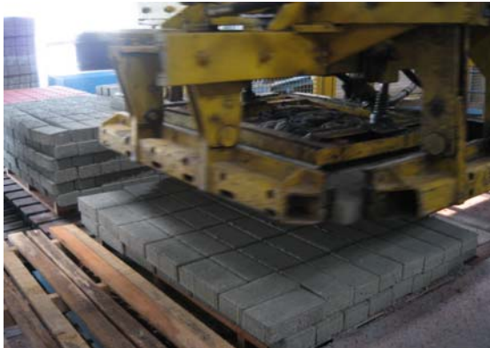
Figure 12: Making a 'cube' of pavers
