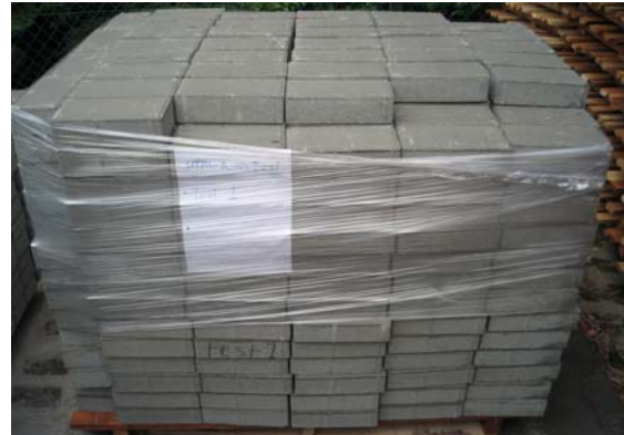
Figure 13: Packed concrete pavers
