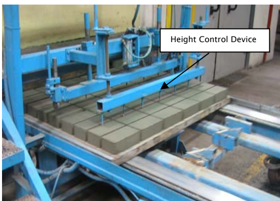
Figure 4: Paver height control
