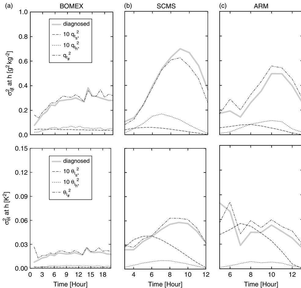
Figure 7. Time series of the diagnosed variances of  $q_t$  and  $\theta_1$  at mixed-layer top (grey), and the corresponding variance scales  $c_{s*}$ ,  $c_{h*}$  and  $c_{\#}$  (black), during (a) BOMEX, (b) SCMS, and (c) ARM. Some scales are multiplied by a factor of 10 for purposes of comparison.
