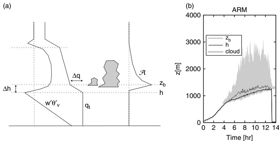
Figure 9. Typical structure of the shallow-cumulus-topped mixed layer. (a) Profiles of the buoyancy flux  $\overline{w'\theta'_v}$ , total specific humidity, and cloud-core fraction  $\mathcal{A}$  (the symbols are defined in the text). (b) Time series of  $h$  and  $z_b$  for the ARM case. The cloud layer is shaded (grey). The transition layer is situated between  $h$  and  $z_b$ .
