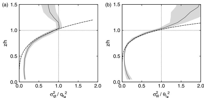
Figure 5. Scaled variance profiles for (a) moisture and (b) liquid-water potential temperature, as in Figures 3 and 4, but averaged over all cases and all hours. The black solid line is the mean, while the grey area indicates the standard deviation. The thick dashed line represents the power-law fit (Equation (8)).
