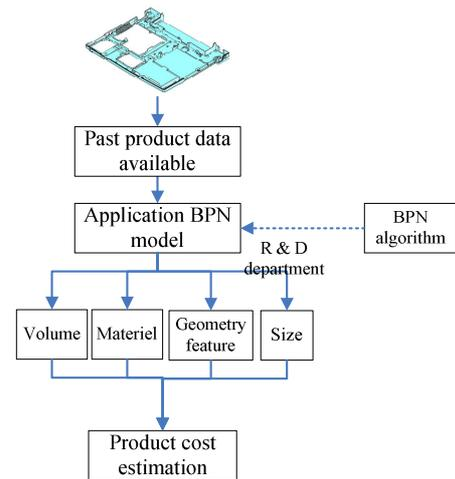
Fig. 4 Technique of estimating plastic injection cost through BPN
