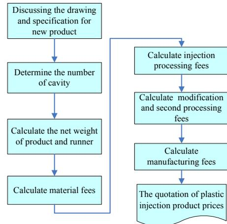
Fig. 3 Cost evaluation procedure for traditional plastic injection industry
