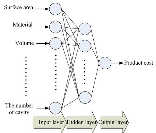
Fig. 5 BPN structure for estimating the cost of plastic injection molded products
